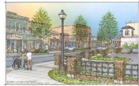
Parking Lots should be set back from the street and must be screened with a low wall
