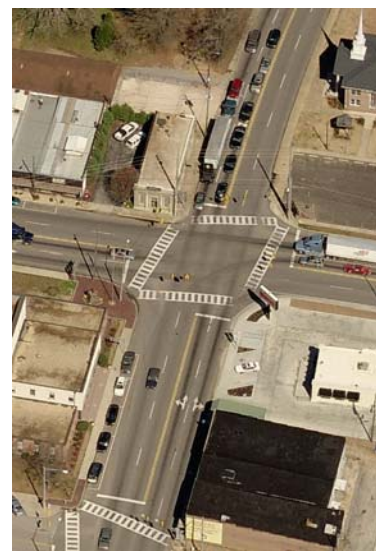
North-south traffic on Military Street (U.S. Highway 43) tends to back up at the intersection with Bexar Avenue (U.S. Highway 278). This may be resolved by adjusting the timing of lights at this intersection and the one immediately south at First Avenue SW.
